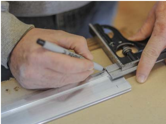
Illustration 59 - Mark rail from end
