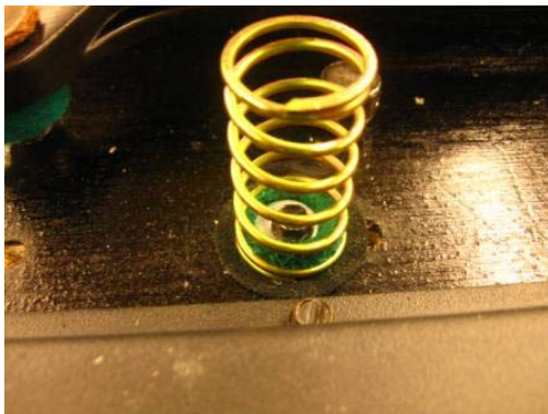
Illustration 108 – Return spring and mounting
