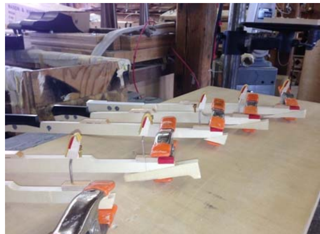
Illustration 12 – Replacing the cut out of the keys
