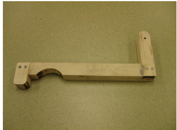
Illustration 102 - Sostenuto lever assembled
