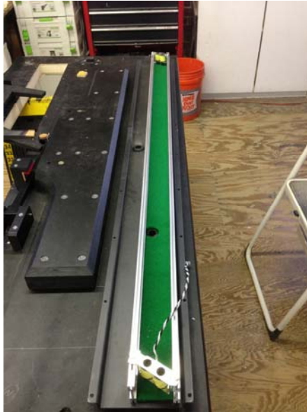
Illustration 118 – Installing key solenoid felt
