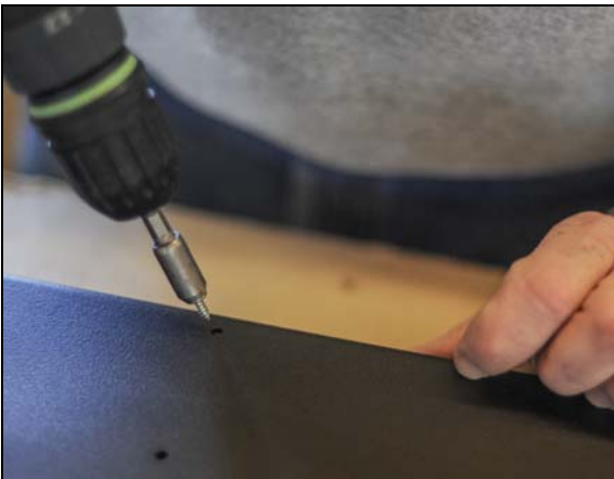
Illustration 67 - Mount solenoid rail on tray
