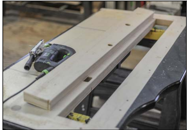
Illustration 54 - Keybed with slot cut
