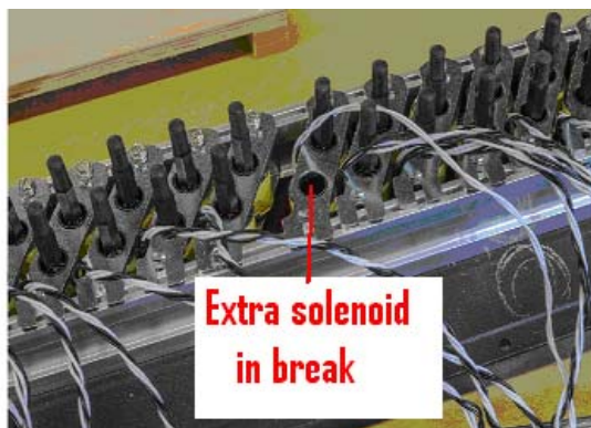
Illustration 21 - extra solenoid in break
