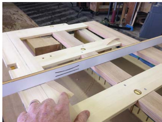
Illustration 27 – Iron-on veneer shim
