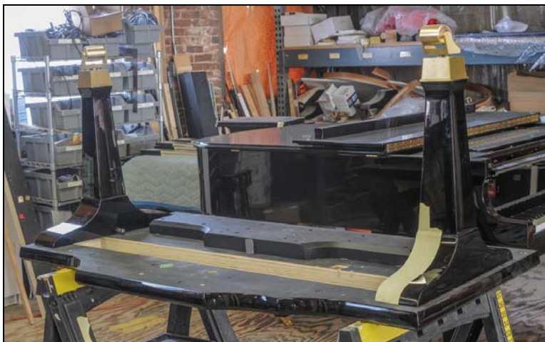
Illustration 55 - Legs attached to keyed off piano
