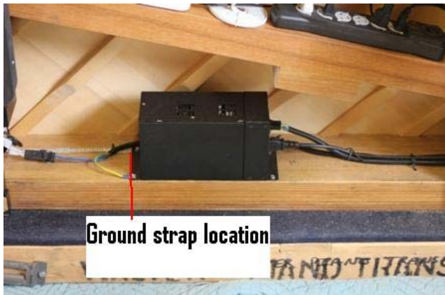
Illustration 135 - 40V Power supply mounted to rim
