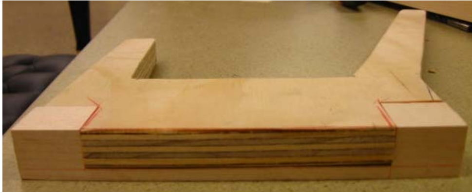
Illustration 91 - Sostenuto lever ready for pivot pins and glide stop
