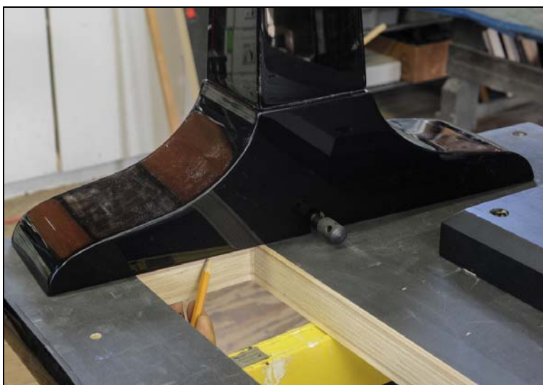
Illustration 56 - Trace slot on leg top
