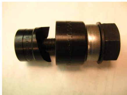
Illustration 85 – Hole punch and Carbide drill for tray hole
