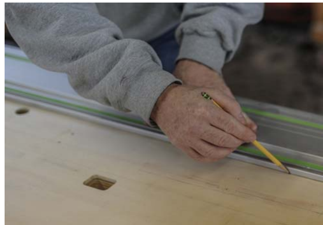
Illustration 46 - Marking back line for slot
