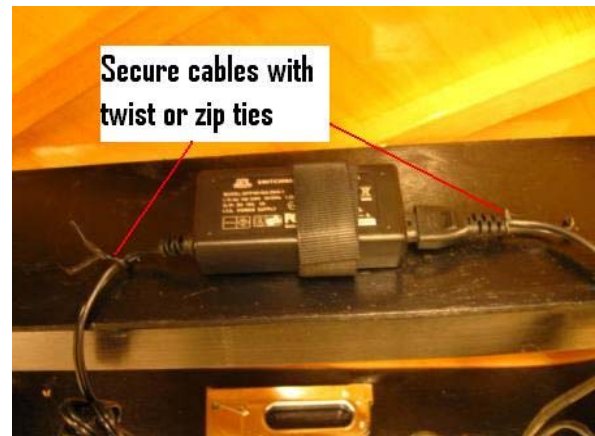
Illustration 136 – 10V power supply on rim
