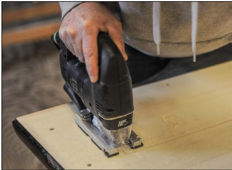
Illustration 50 - Cut ends of slot
