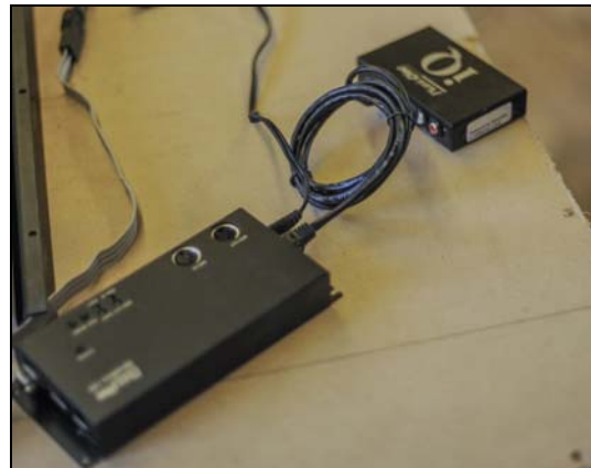
Illustration 129 - Connecting data to iQ box
