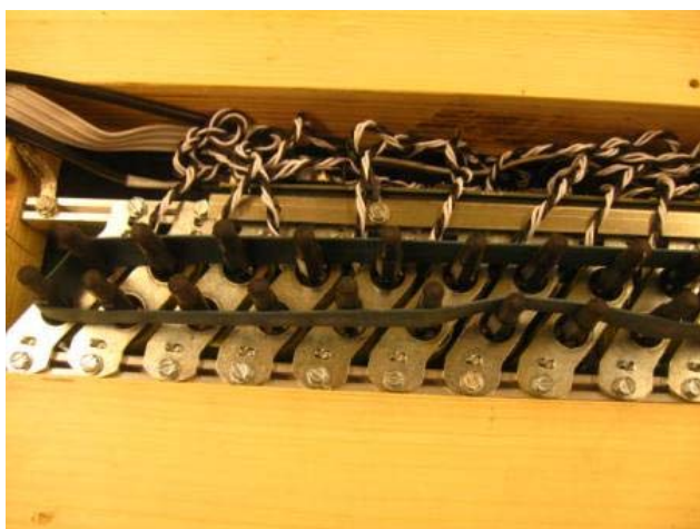
Illustration 140 – Securing key solenoid plunger with rubber band
