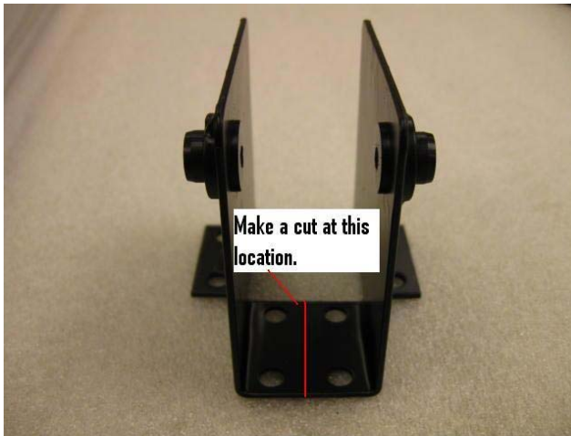
Illustration 92 – Trapwork bracket cut in half
