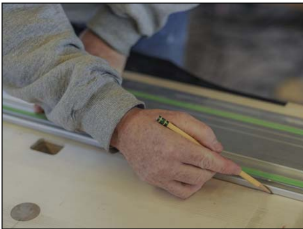
Illustration 45 - Marking front line for slot
