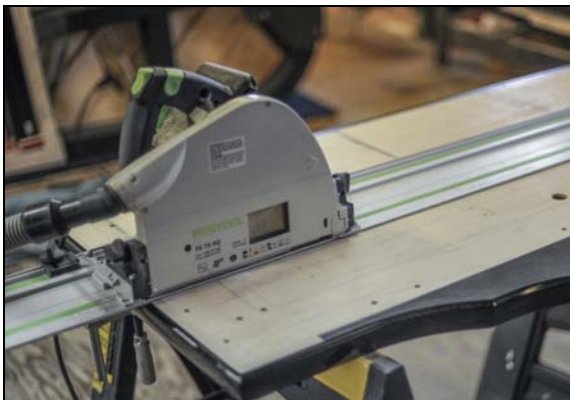
Illustration 51 - Cutting front of slot
