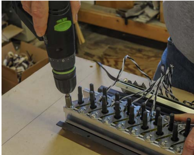
Illustration 119 - Mount solenoid pairs on rails
