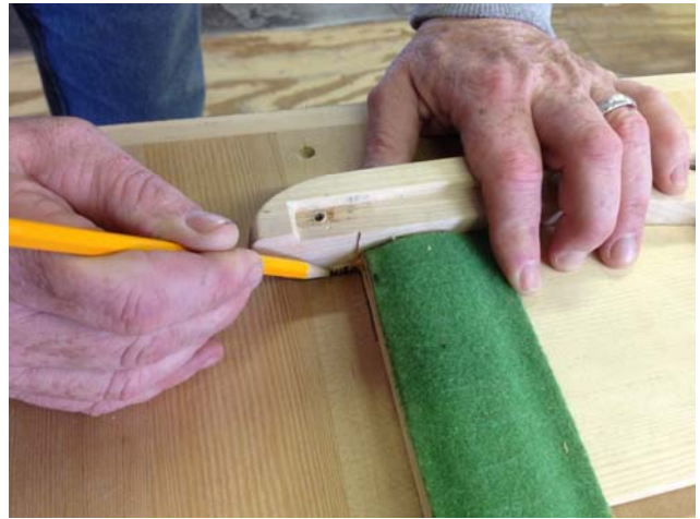
Illustration 40 - marking keyframe cut on keybed
