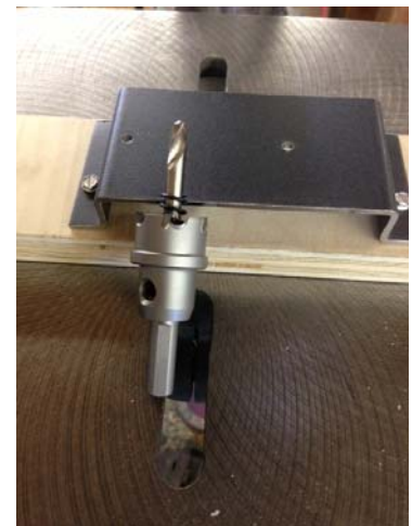
Illustration 85 – Hole punch and Carbide drill for tray hole
