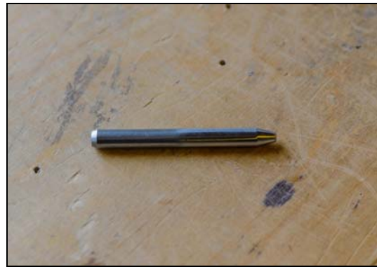
Illustration 10 - WNG stainless steel locating pin
