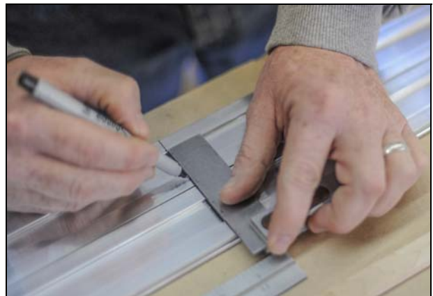
Illustration 62 - Marking cut line on rails
