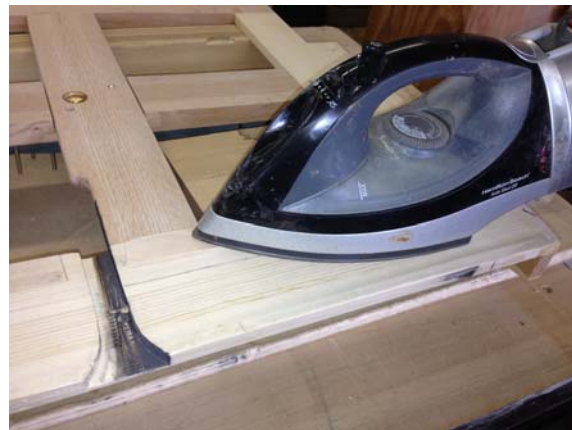
Illustration 29 - Ironing on veneer
