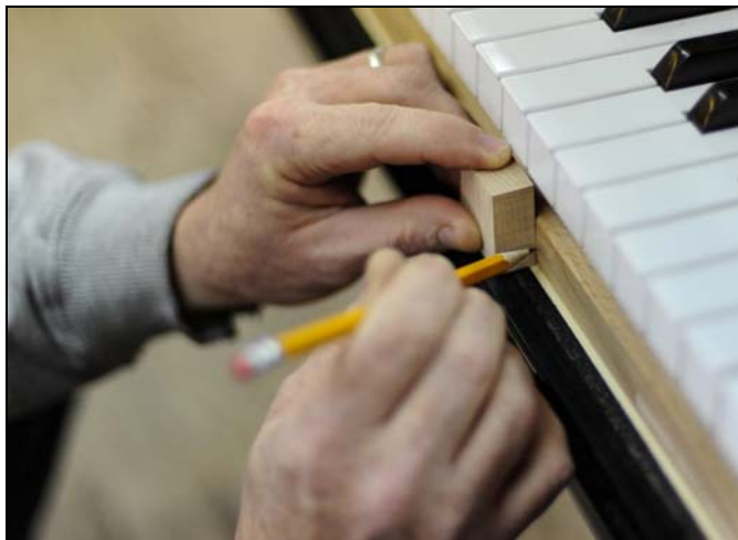
Illustration 2 - Marking front of keyframe
