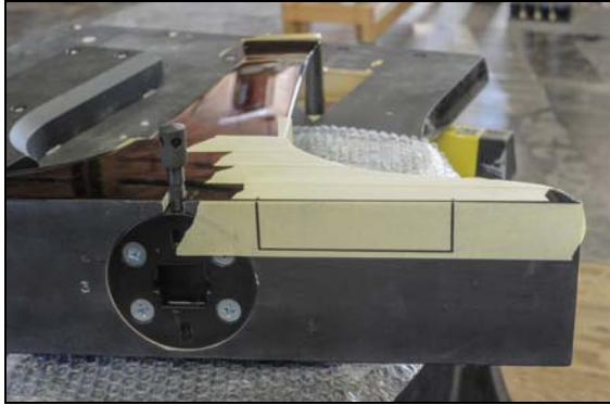
Illustration 57 - Mark cut on top of leg
