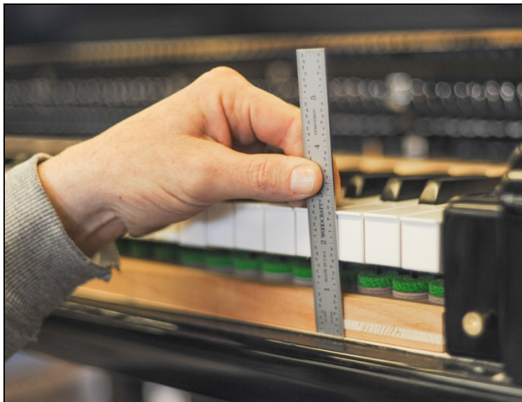
Illustration 4 - Measuring key height - front
