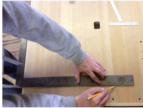
Illustration 48- Marking end slot cut
