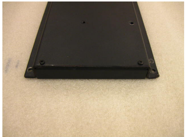
Illustration 117 – End cover plate installed
