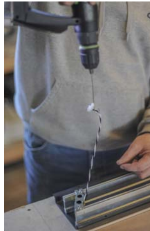
Illustration 123 - Twist solenoid wires
