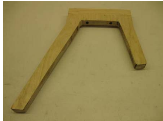
Illustration 88 – Optional butt joint connection
