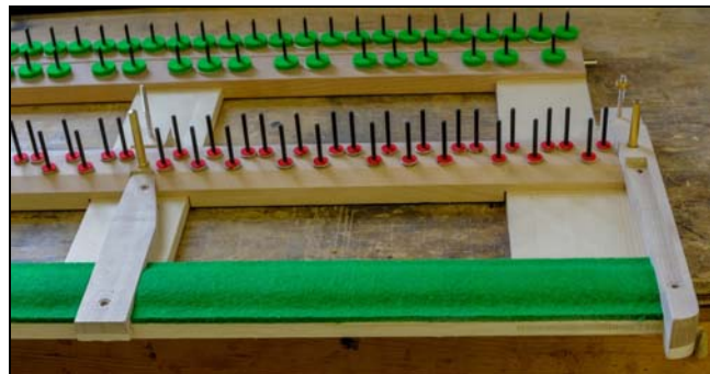
Illustration 32 - cleats extending behind the back rail
