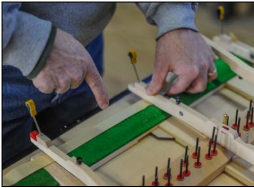
Illustration 23 – Marking keyframe cut location
