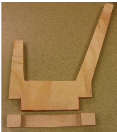
Illustration 89 - Lever with hardwood addition
