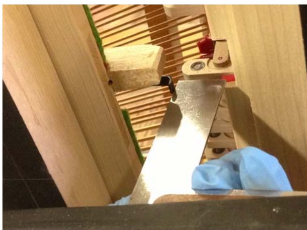
Illustration 3 – Locating the pitman to lever
