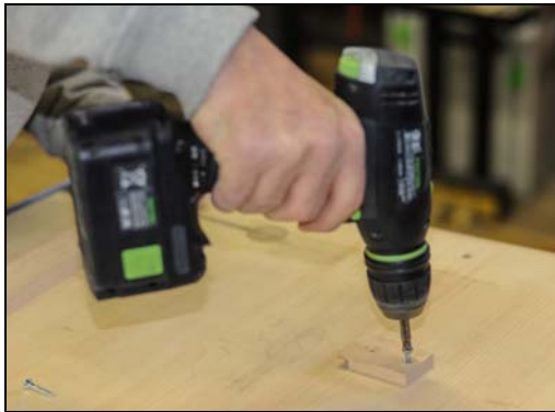
Illustration 35 - Remove dag screws
