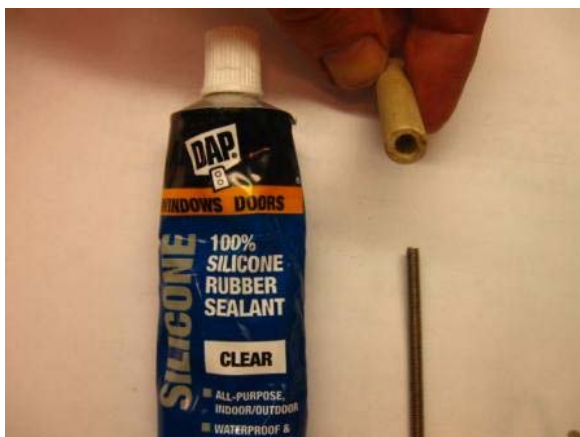
Illustration 7 & 8 – Pitman rod glued into dowel
