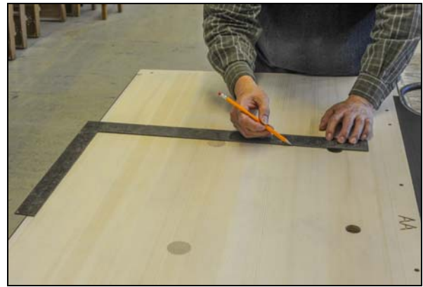
Illustration 16 - Mark Sostenuto pitman hole
