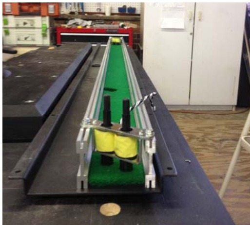
Illustration 69 – Installing bass solenoid assembly
