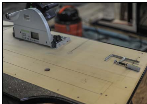
Illustration 52 - Front and back cuts for slot
