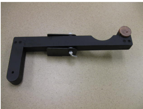
Illustration 103 - Finished sostenuto lever
