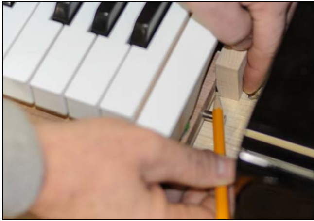
Illustration 3 - Marking side of keyframe
