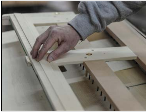
Illustration 30 - Back rail shim, soft wood
