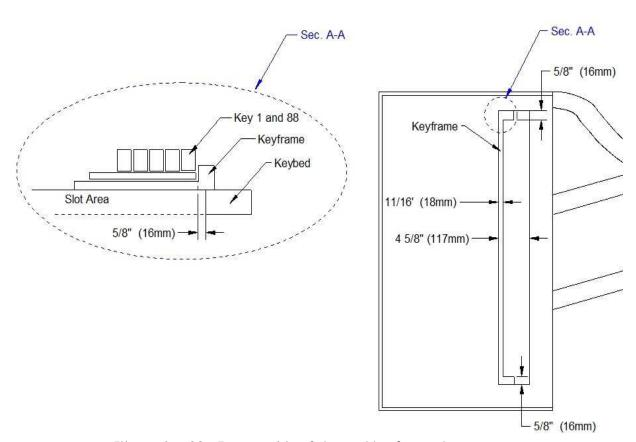
Illustration 38 - Bottom side of slot and keyframe dimension
