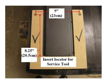
Illustration 4 – Jig for installing tool inserts
