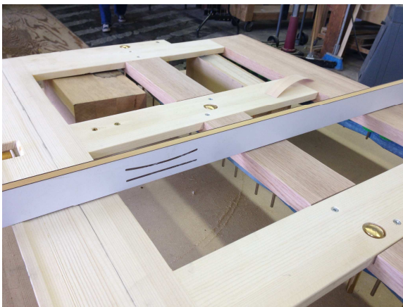
Illustration 26 – Keyframe without support bead
