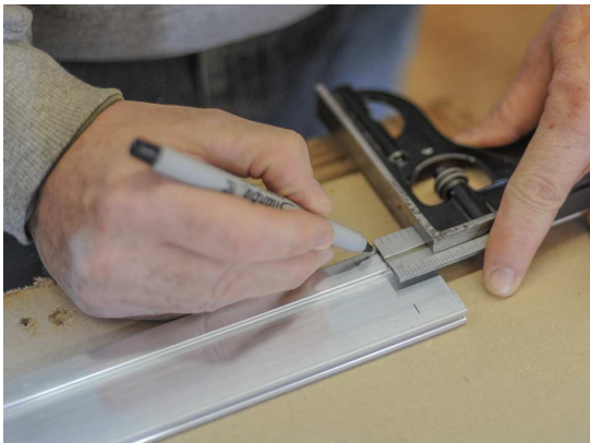
Illustration 55 - Mark rail from end
