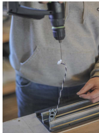
Illustration 125 - Twist solenoid wires
