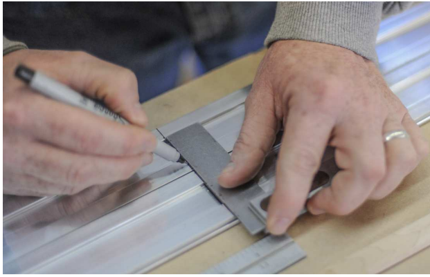
Illustration 57 - Marking cut line on rails
