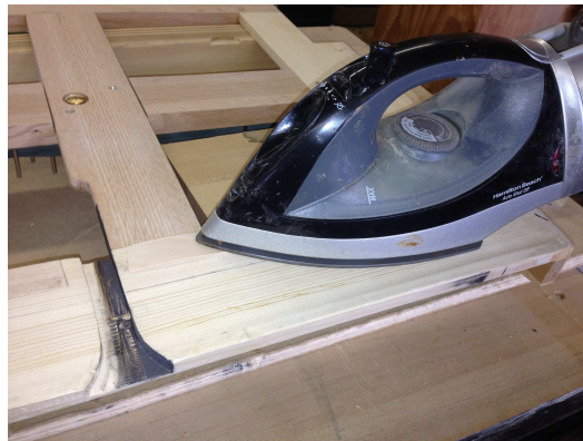
Illustration 29 - Ironing on veneer
