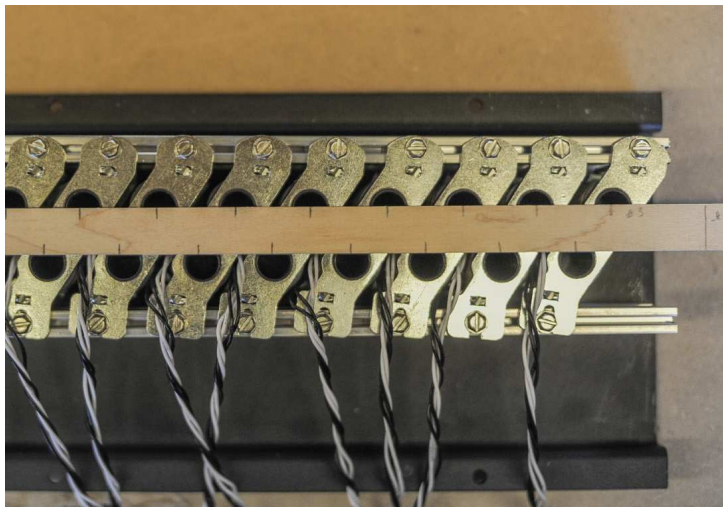
Illustration 122 - Use scale stick to locate solenoids
