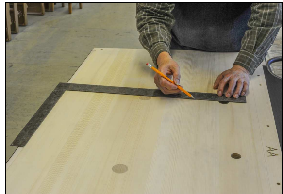
Illustration 16 - Mark Sostenuto pitman hole
