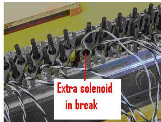
Illustration 21A - extra solenoid in break
