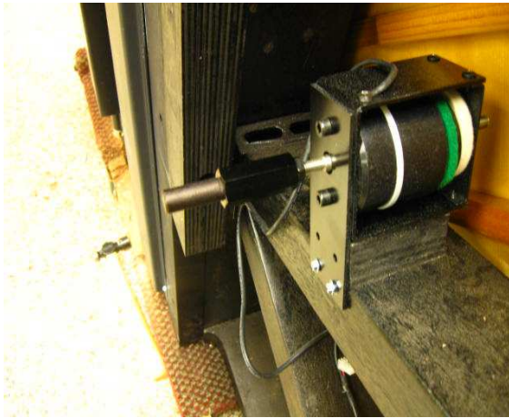
Illustration 74 – Mounting pedal solenoid
