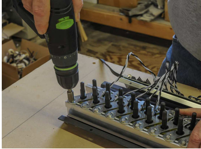
Illustration 120 – Installing key solenoid felt Illustration 121 - Mount solenoid pairs on rails
