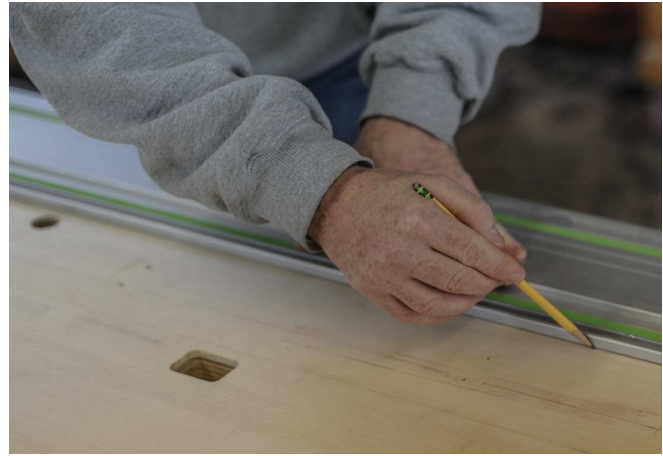
Illustration 46 - Marking back line for slot
