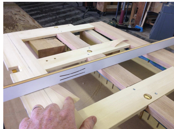
Illustration 27 – Iron-on veneer shim
