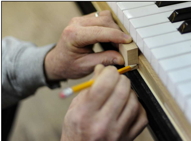
Illustration 2 - Marking front of keyframe
