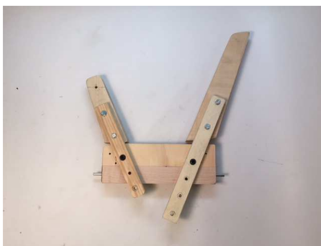
Ill. 90 – Adjustable sostenuto jig (push type)
