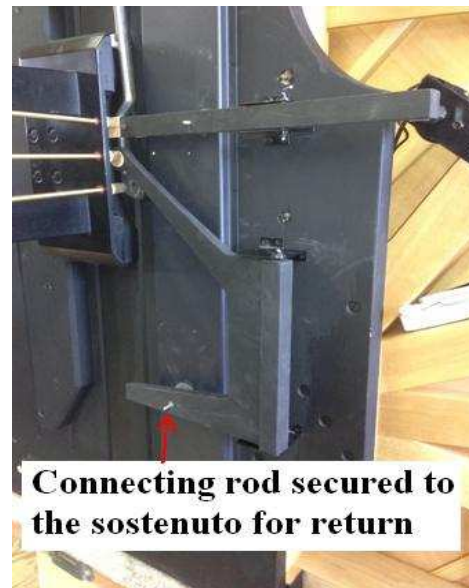
Illustration 97 - Sostenuto lever installed
