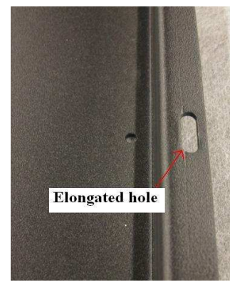
Illustration 65A – Elongated screw holes
