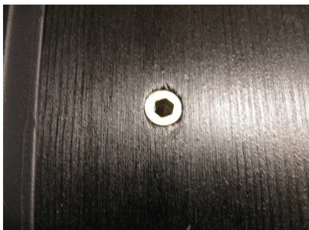
Illustration 69 – Insert installed into Keybed
