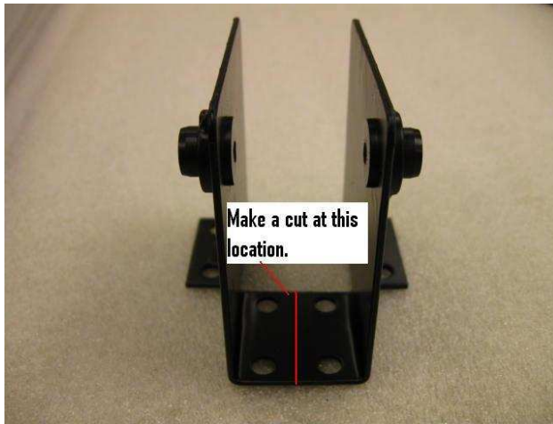
Illustration 93 – Trapwork bracket cut in half
