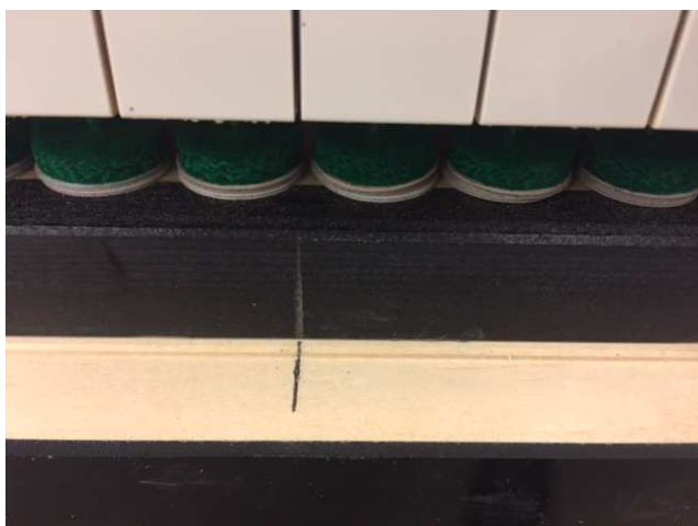
Ill. 39 – Align action with previous marks, front and side
