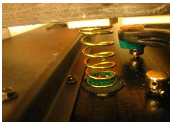
Illustration 110 – Return spring finished
