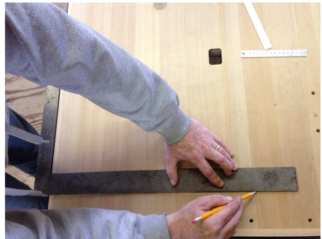
Illustration 48- Marking end slot cut
