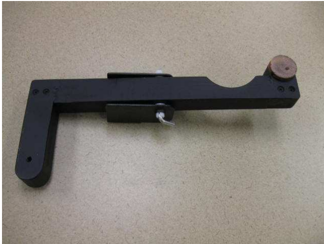
Illustration 105 - Finished sostenuto lever
