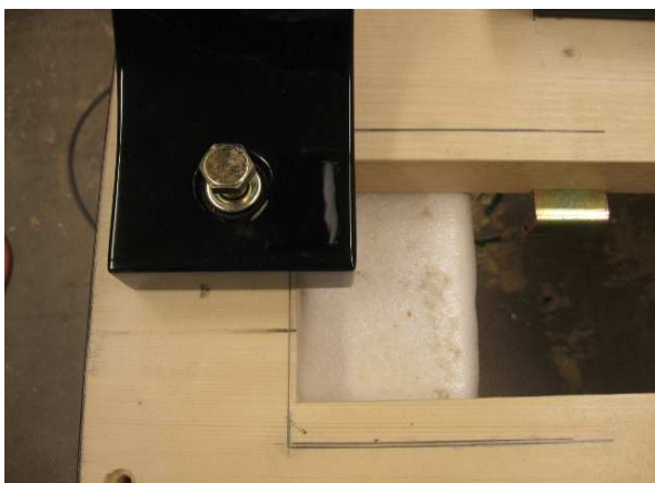
Illustration 70 - Legs attached to keybed
