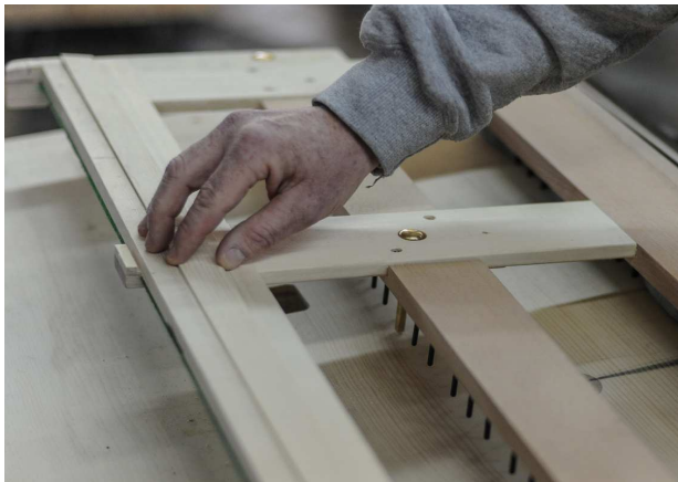
Illustration 30 - Back rail shim, soft wood
