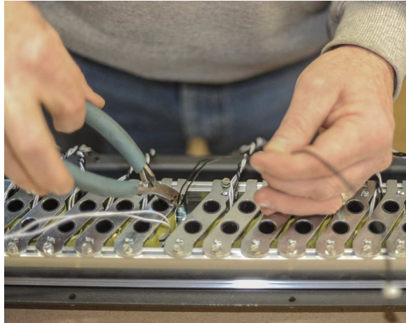
Illustration 123 - Cutting wires on unused solenoids.
