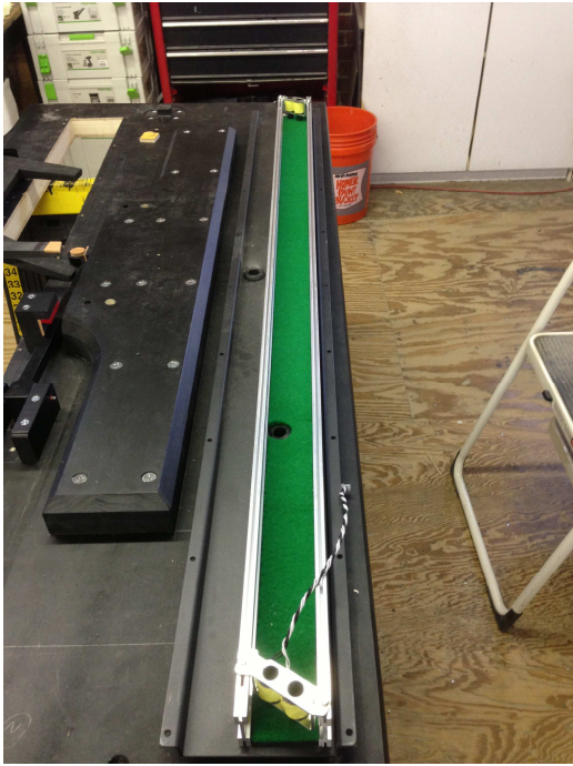
Illustration 120 – Installing key solenoid felt Illustration 121 - Mount solenoid pairs on rails
