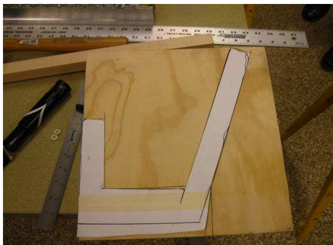
Illustration 89 - Sostenuto Pattern on plywood
