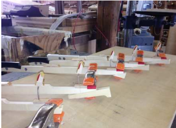
Illustration 10 – Replacing the cut out of the keys
