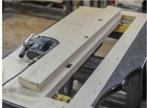
Illustration 54 - Keybed with slot cut
