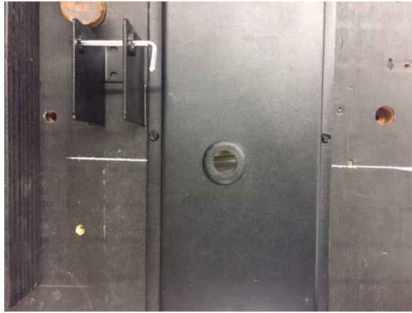
Illustration 87 – Sostenuto hole drilled with grommet in place
