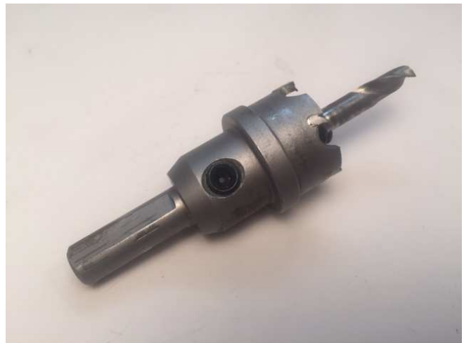
Illustration 86 – Carbide drill for tray hole
