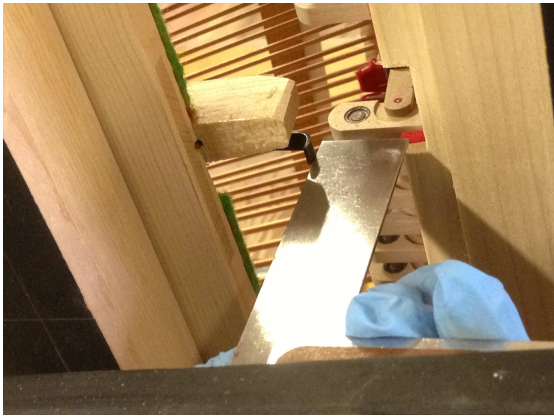
Illustration 5 – Locating the pitman to lever
