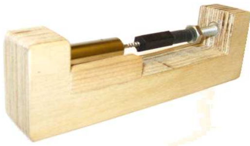
Illustration 114 – Key Plunger Tool
