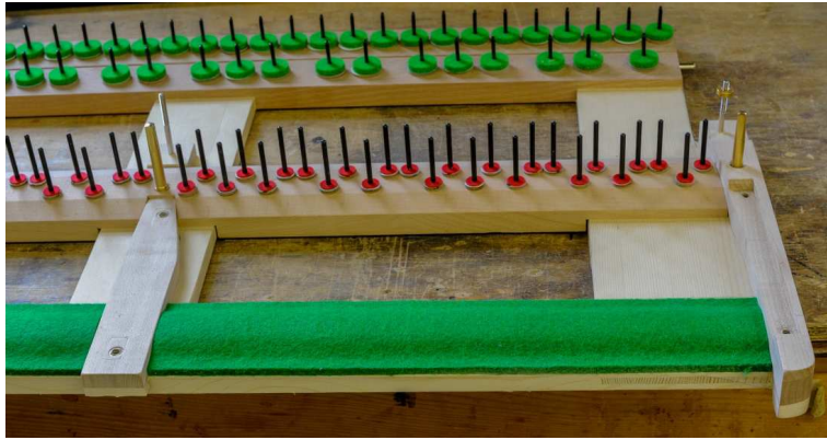
Illustration 32 - cleats extending behind the back rail
