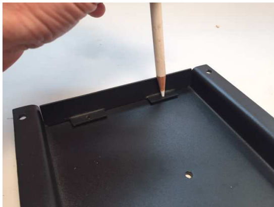
Illustration 62 – Mark end plate holes
