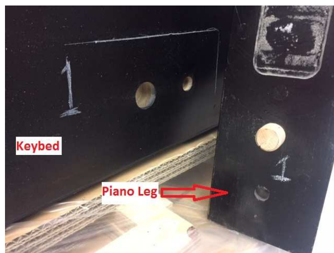
Illustration 8A – Mark leg location
