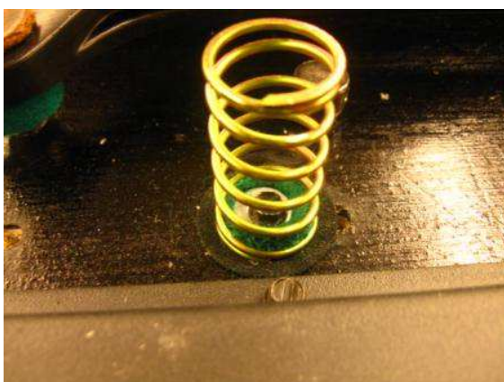
Illustration 109 Return spring installed
