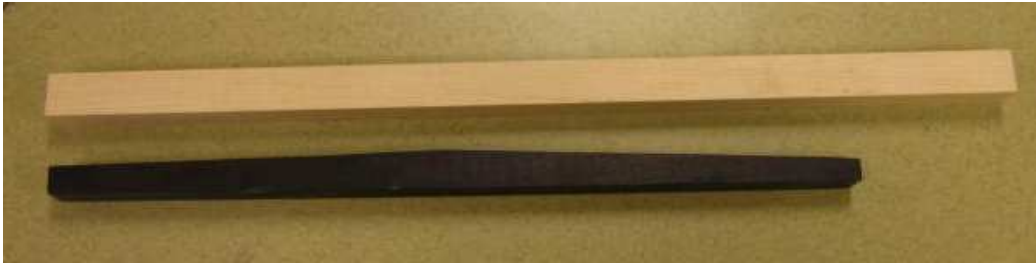
Illustration 76 – finished and unfinished sustain lever
