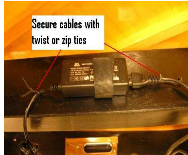
Illustration 138 – 12V power supply on rim
