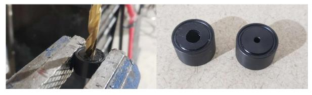
Step 5: drill a hole for the locking screw.
