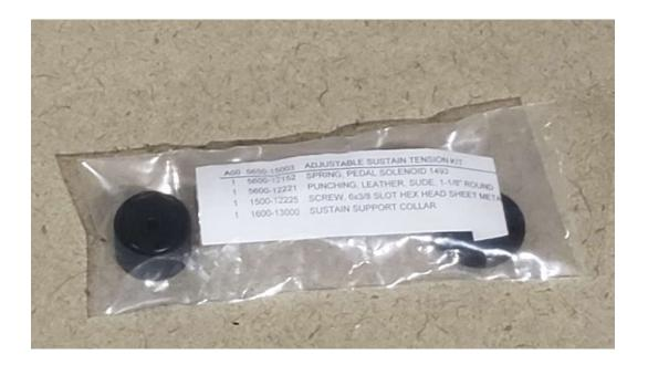
The adjustable sustain tension kit allows for an increase in spring tension in any grand piano. It is often the case that installing a player system on a piano may decrease the tension of the sustain pedal. This is often a requirement due to the fact that the pedal solenoid requires the minimum amount of tension to ensure it doesn't overheat. This kit allows you to add the spring tension back to any pedal by placing the spring on the lyre.
