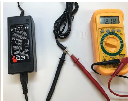
Checking small power supply
