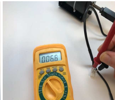
Testing ohm resistance
