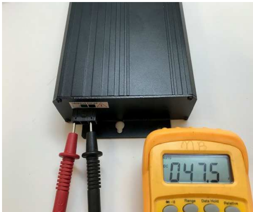
Checking large power supply
