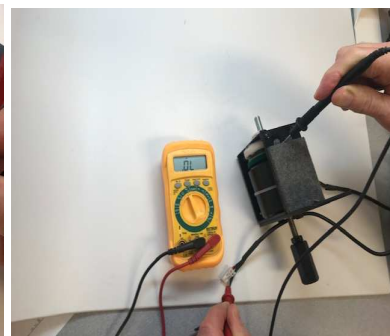
Checking for grounding
