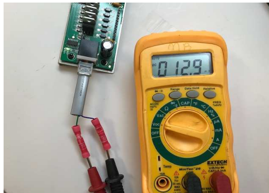
Checking power out of key driver board
