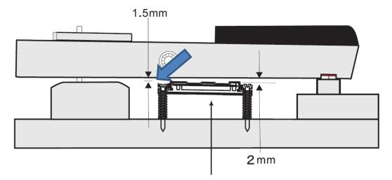
3. Place the key sensor rail as high as possible to the key bottom when pressed. It's well placed just if you don't hear the touching sound of sensor rail and key bottom.
